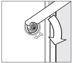
■ Turn the right shipping strut counterclockwise 90° with the enclosed combination wrench and.
